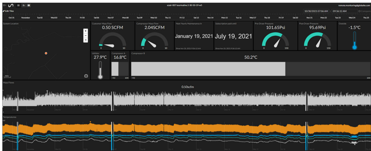
Figure 16 - EZ Air 2hp with M5 screenshot from Initial State (remote monitoring)
