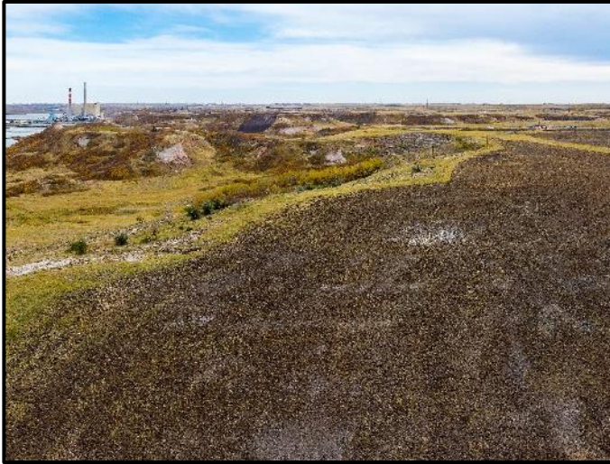
Photograph 1: Biosolids were applied and incorporated to amend over 800 ha of land at Paintearth Mine. This included historically reclaimed land that did not meet current reclamation standards. (August 2019)
