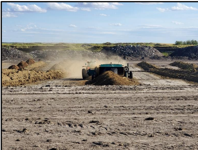
Photograph 3: Operational testing of the Frontier Soil Turner, one of the tested mixing techniques for the subsoil blend and extend activity. (September 2021)
