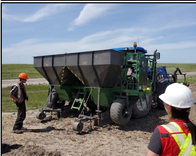
Photograph 5: The BIOSALIX willow billet planters, the first of their kind in North America, were piloted for the project. This planter lays the willow billets flat in the base of a furrow which is then covered with soil. (May 2021)
