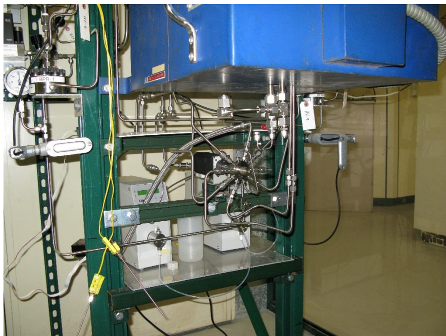
Figure 4. Picture of the 10-port valve and associated tubing.
