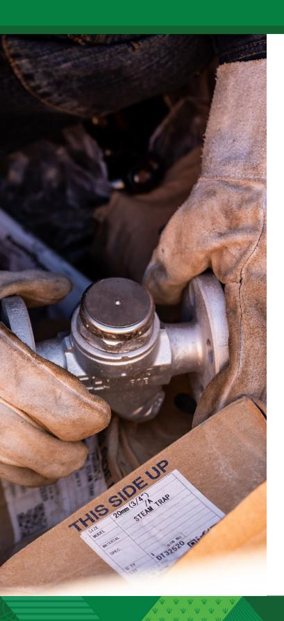
Have you inspected your steam distribution system recently? Steam traps should be checked regularly for leaks and proper performance. It's common for steam trap leaks to go undetected and, if not properly inspected, could result in additional natural gas costs of over \$1,000 per year.
