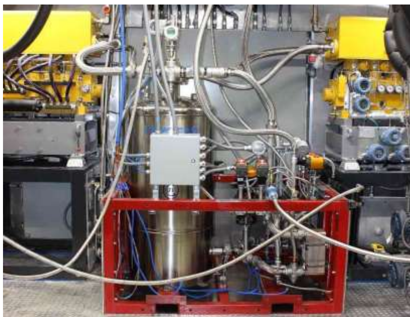
Figure 8. Installed energy storage system (i.e., LNG cold box).
