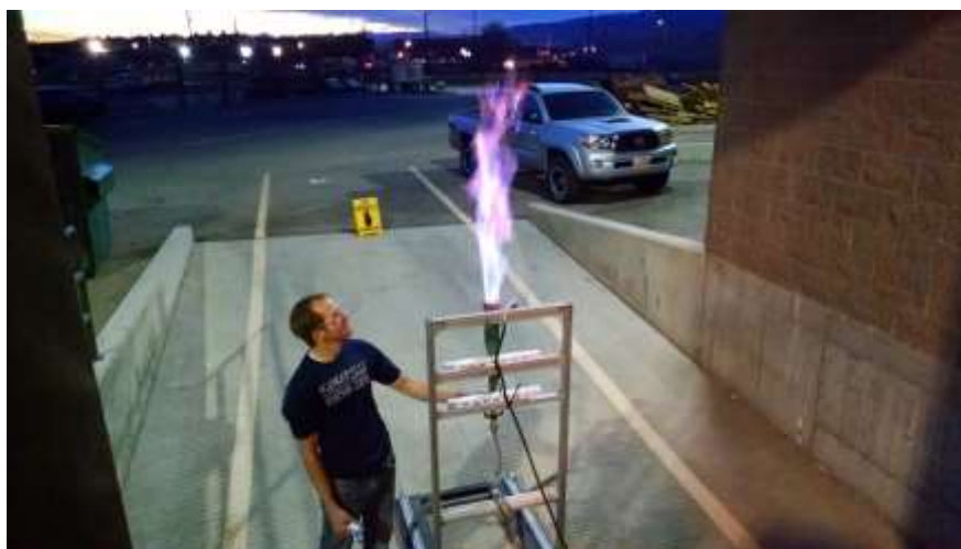
Figure 25. Adjusting the fuel/air mixture while flaring natural gas after it was used in its condensed phase (LNG) to drive the CCC process.
