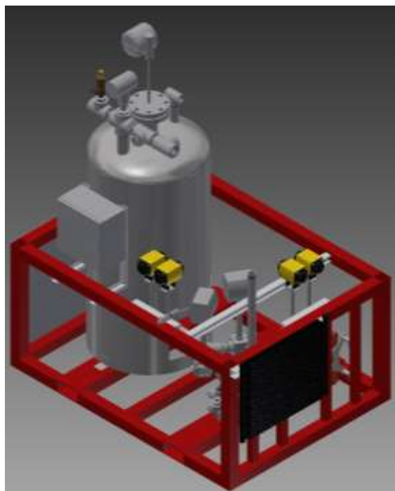
Figure 7. LNG cold box CAD design (all hose runs removed).
