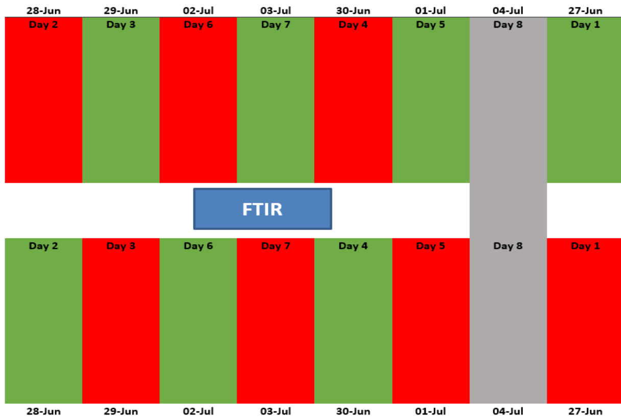
Fig. 29. The schedule of CH 4 observations over an eight day period. Low RFI FAT cattle are depicted by the green strips and high RFI FAT cattle are depicted by the red strips on either side of the OP-FTIR unit. Strips are not shown to scale. Cattle were adjusted to strip-grazing on day one and CH 4 measurements were not collected.
